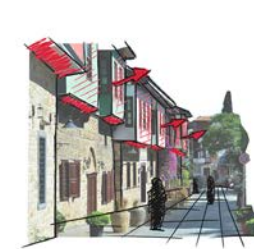
Over hangs on 2nd floors for more spaces, 1st floor is masonry stone while 2nd floor is timber. Change in use of materials and forms.
