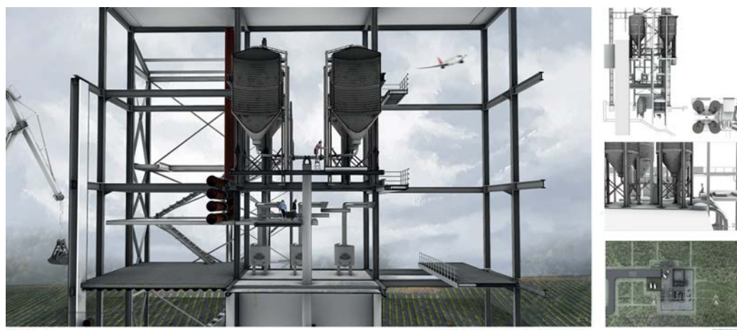
SECTION AA FROM MATERIAL FLOW TO SPATIAL IMPACT Grain storage > Malt mill > Brew House > Cooling Block > Fermentation > Packaging > Storage/Delivery
